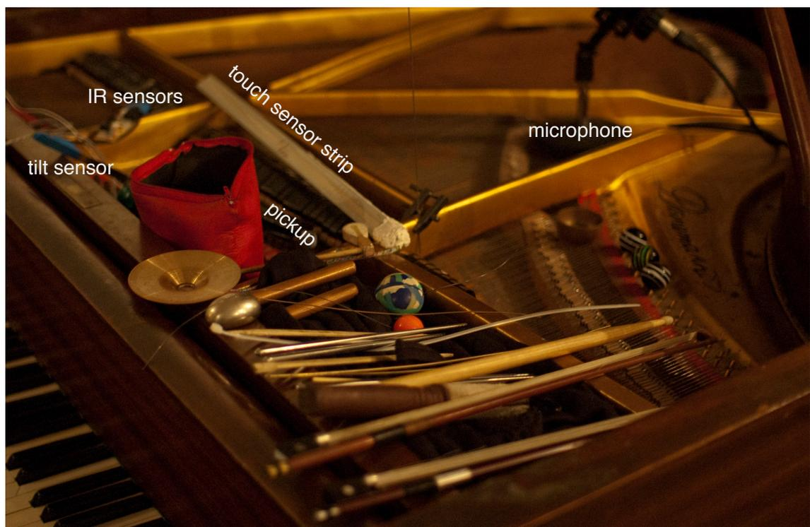
Figure A14: *piano+* preparations, tools and sensors
