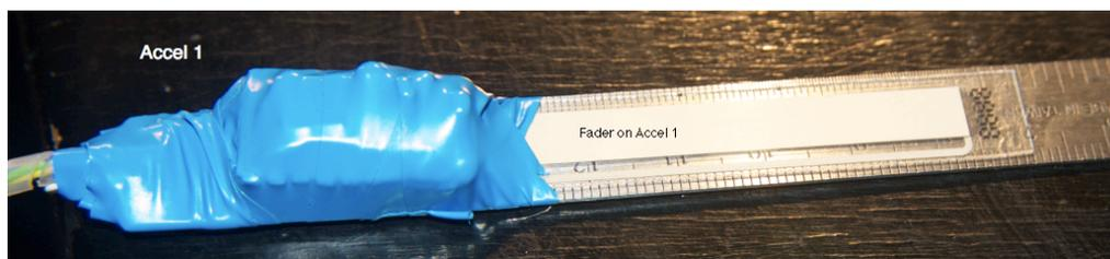
Figure A15: tilt sensor Accel 1 mounted on a metal ruler with an additional touch sensor strip. Acceleration sensors ADXL335 , Touch sensor strip.
