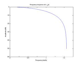
**Figure 2.** The frequency response of the Haar approximation component  $A_1(z)$ , a simple lowpass filter. Above,  $F_s = 2\pi$ . Therefore, the maximum frequency component is equivalent to  $F_s/4$ , half the Nyquist frequency due to downsampling.
