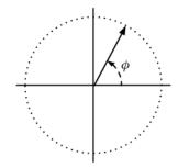
Figure 2: A metronome ticking at f bpm is represented as a phasor which rotates  $2\pi$  radians once every  $T=\frac{60}{f}$  seconds. For any time t, the current phase  $\phi$  is the fractional portion of  $\frac{t}{T}$ .
