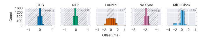
Figure 7: Histograms of the offset data, along with  $\sigma$ , the standard deviation for each. Note that the x-axis range is not the same for each plot. The hatch-shaded area indicates a 2 ms range centered on each mean. GPS offers the most accurate synchronization, followed closely by NTP, while MIDI clock and LANdini exhibit similar performance. "No Sync" has low standard deviation, but is offset by -2 ms.
