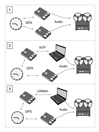
Figure 4: We tested 3 configurations of PIGMIs along with two "control" configurations (shown in Figure 5) in order to learn the magnitude of synchronization error. In each of the displayed configurations, we recorded 30 minutes of audio ticks at f=120 beats per minute. Then, we analyzed the per-tick timing differences (offsets) of one recording compared to the other.
