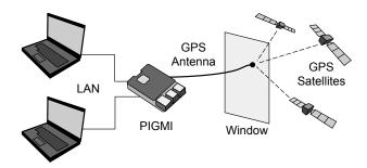
Figure 3: The Pi Global Metronome Implementation (PIGMI) is inexpensive and portable, and greatly simplifies the process of synchronizing to the Global Metronome. It requires a view of the sky in order to sense GPS satellites. To use it, place its antenna in a window, and connect the PIGMI to a network.
